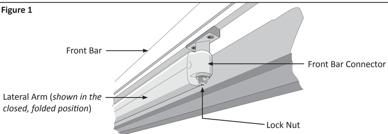
**Note:** The two Front Bar Connectors attach each Lateral Arm, left and right, to the Front Bar.
